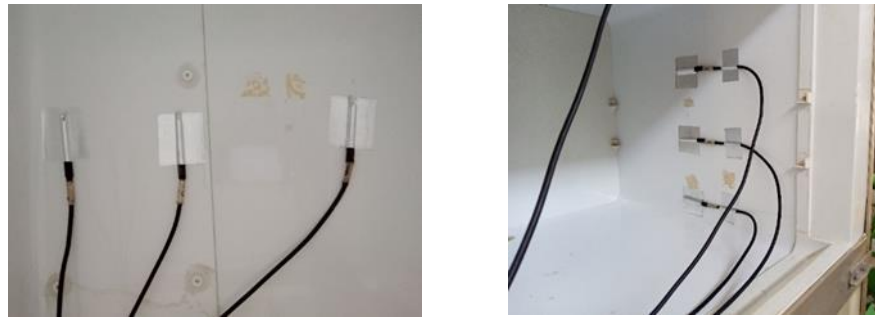
Figure IV. Placement of temperature sensors at compressor dome
