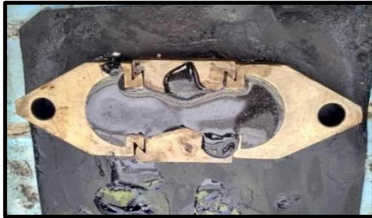
Figure II. Ductility Sample.
