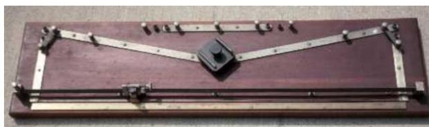
Figura V. Puente Wheatstone (Leeds and Northrup).
