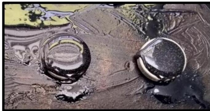
Figure III. Softening Point Sample.
