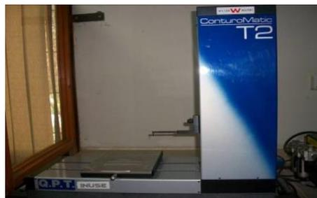
Figure V. Surface Roughness Tester WW CM T2.
