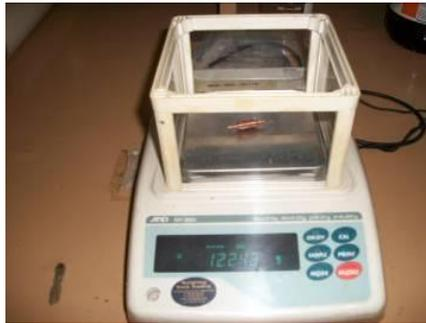
Figure IV. Precision weighing scale AND GF-200.
