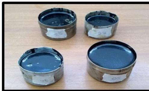
Figure I. Penetration Sample.
