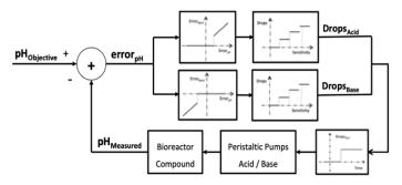
Figure X.- Block diagram of proposed pH ON-OFF control
