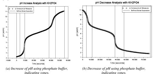
Figure. IX.- Results of continuous evolution of pH values in work range
