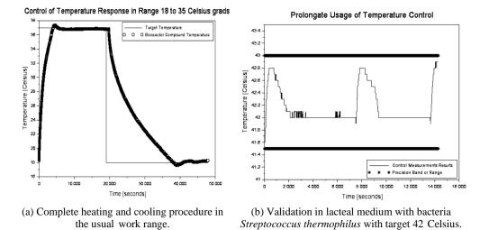
Figure VIII.- Application and testing of proposed temperature control
