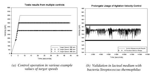
Figure IV.- Application and testing of proposed agitation velocity control
