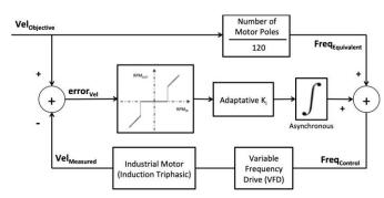
Figure III.- Block diagram of proposed Agitation velocity control
