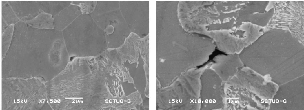
Figure 11: Decohesions or microcavitations between the ferrite and pearlite during superplastic deformation (R-shaped crack) (a) and as a consequence of a conventional high-temperature deformation (decohesions between matrix and hard constituent) (b).
