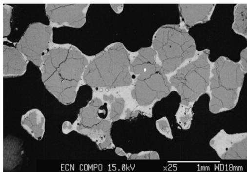
Figure IV.- Agglomeration of solid ash particles due to lower melting point salts [3]
