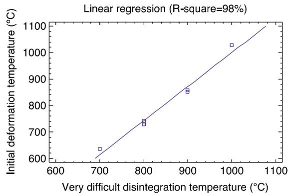
*Figure V.- Correlation between initial deformation temperature and sintering test evaluation [4]*
