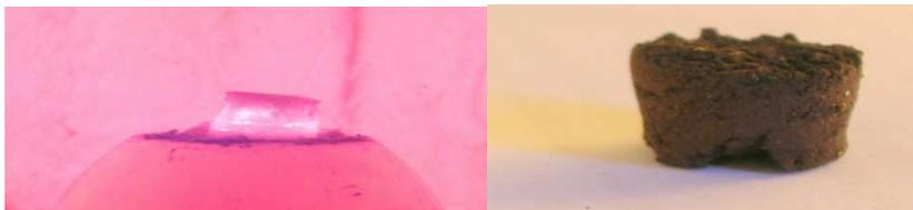
*Figure IX.- (a) Ash sample in furnace (b) Sintered sample after exposure to 900C*
