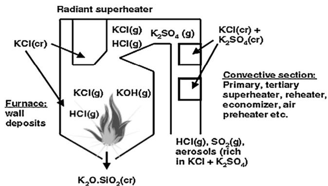
Figure III.- Principal pathways of K, P and Cl in a biomass fired boiler [3]
