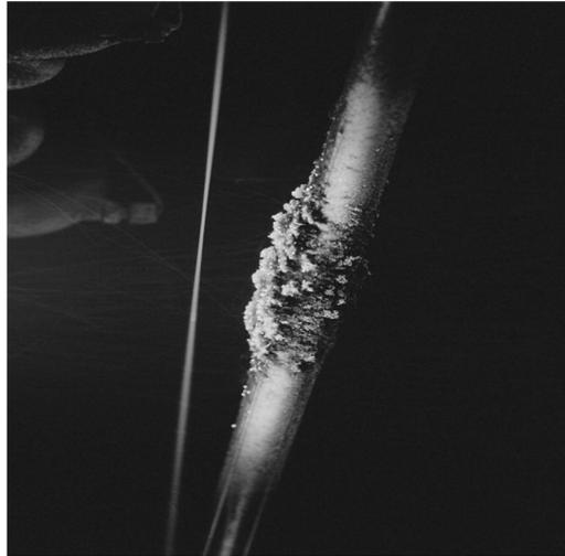
Figure II.- Photograph of deposit forming from wheat straw on a simulated boiler tube [3]
