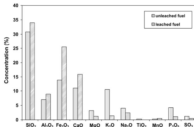
Figure VI. Main components of fly ashes of leached and unleached olive kernels [14]
