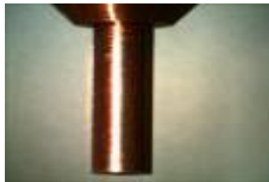
Figure II. Copper Electrode Tip at 17 X prior to Machining.
